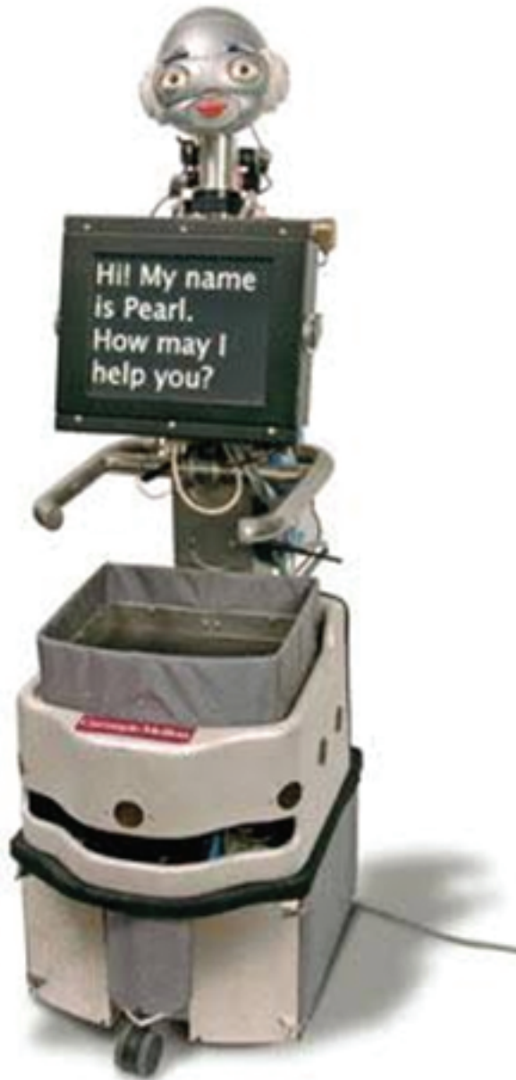
Fig. 6: Pearl is an interactive assistant robot for the elderly
