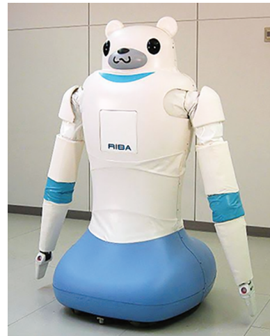
Fig. 5: Robot for interactive body assistance (RIBA) is a robotic nurse that can lift a patient and move them to another location
